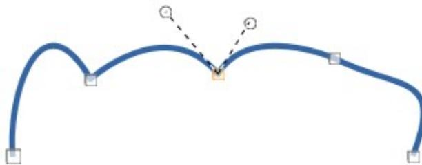
Figure 300: Example of a corner point
