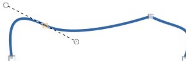
Figure 301: Example of a smooth transition point
