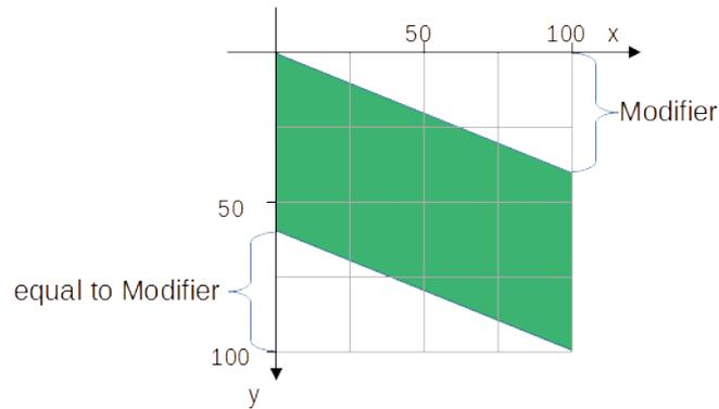
Figure 30: height of parallelogram = height of snap-rectangle
