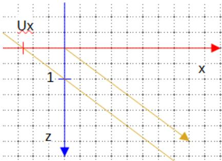
First, we look at the 3D-scene from top to bottom. The grid has 0.5 line spacing. For this view we need only the x-coordinate and the z-coordinate. The yellow arrow is the projection direction. The yellow straight line is parallel to the projection direction. This line meets the xy-plane in the x-coordinate  $U_x$ .
