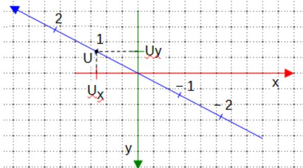
As last step, we look on the 3D-scene from front to back and identify the point  $U(U_x|U_y)$ . In fact, we get not only the point  $U$ . We get the whole image of the z-axis and a scale on this image.
