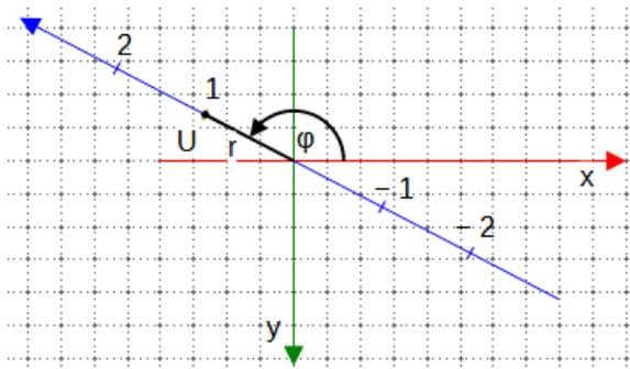
The angle  $\varphi$  is positive in the shown direction.
