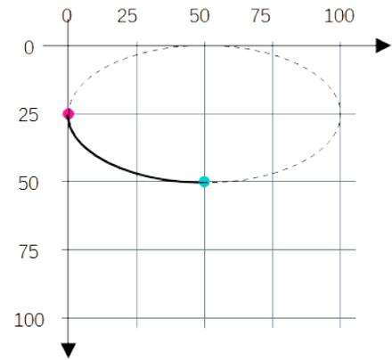
Figure 32: Elliptic arc with 90deg center angle
