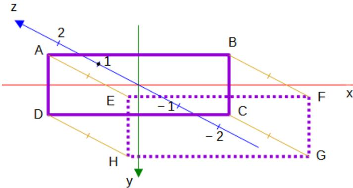
The solid purple rectangle is the front face, the dotted one is the back face. To get the point E, take a copy of the segment from 0 to -2 of the image of the z-axis and move it to the point A. Do the same for all points of the front face.
