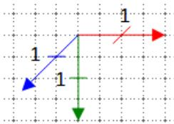
To use a coordinate system as shown in the illustration, you need to set `draw:skew="70.71 -135"`. Using a skew angle  $-135$  results in a projection, where those lines, which go from the observer perpendicular to the  $xy$ -plane are drawn with a  $45^\circ$  angle to the  $x$ -axis. The reduction factor of  $70.71 \triangleq \sqrt{0.5} \approx 0.7071$  corresponds to the length of the diagonals in a grid square.
