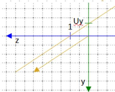
Now we look at the 3D-scene from right to left. For this view we only need the y-coordinate and the z-coordinate. The yellow arrow is again the projection direction. Again we construct a parallel straight line through the unit point of the z-axis. It intersects the xy-plane in y-coordinate  $U_y$ .
