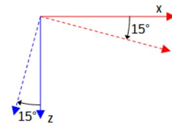
We apply both rotations, first the rotation around the y-axis, then the rotation around the x-axis. So we get the total matrix
