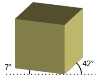
The “isometric” projection needs a rotation of  $45^\circ$  about the  $y$ -axis and a rotation about the  $x$ -axis of about  $35^\circ$ . The cube in the illustration has the markup
