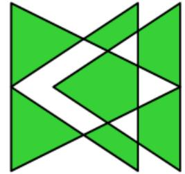
Figure 41: Example even-odd filling rule
