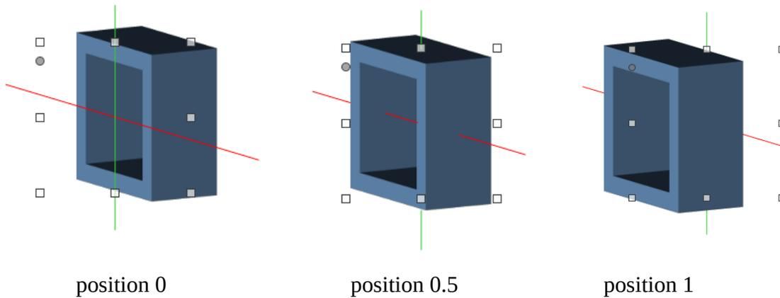
Figure 113: Rotated shape with different extrusion positions
